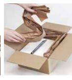
The converter forms single layer kraft paper into a high volume star-shaped paper configuration, which can be used as an effective filling material. It prevents products from shifting around in their box, ensuring damage-free arrival at the end destination. The converted paper gets dispensed directly at the point of operation, improving the efficiency of the packaging process and optimizing the speed of working.
